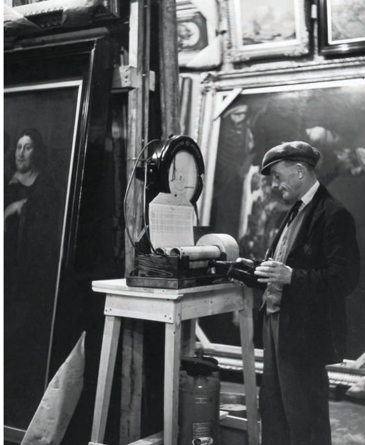
An attendant examines a recording thermohygrograph in a subterranean chamber at Manod Quarry, north Wales, where paintings from London’s National Gallery were moved for safekeeping during World War II. Experiences like these increased understanding of the effects of indoor climate on vulnerable materials. Photo: Fred Ramage/Keystone Features/Hulton Archive/Getty Images.
